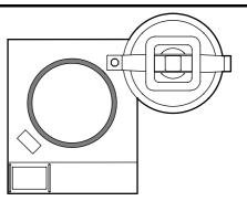
The gasket may deteriorate according to use. If steam escapes frequently, you may need to change the gasket.
