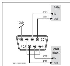
Every B-S balance is fitted with an RS232C interface for attachment to a peripheral device (e.g. printer or PC with a 9-pin male connector). Matching to a different device can be carried out in the menu (Sections 4.3.10 – 4.3.15).
